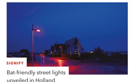
The first street lights designed to be friendly to bats were installed in a town in Holland in June 2018. A partnership between UK-based lighting company Signify, the University of Wageningen, and the municipality of Nieuwkoop, the scheme uses smart LED lights which emit a red color and use a wavelength that doesn't interfere with a bat's internal compass. Remote management of the lights also allows them to be dimmed through the night.
